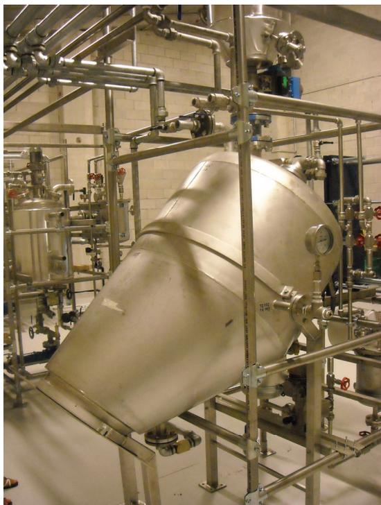
**Fig. 1.** Steam explosion pilot plant
