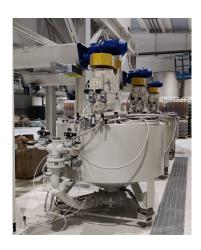
• The Perissinotto Powder Dissolver was designed to create a density-controlled liquid solution out of any type of dust soluble in water or other liquids. Its applications range from dust coming from dust filters, hydrocyclones on spray dryers, colored oxides, and recycled dusts.
