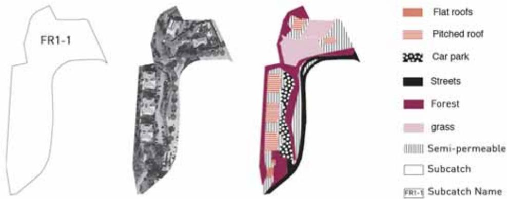
Fig. 5. Example of the investigation process of permeability that was made for each sub-catchment
