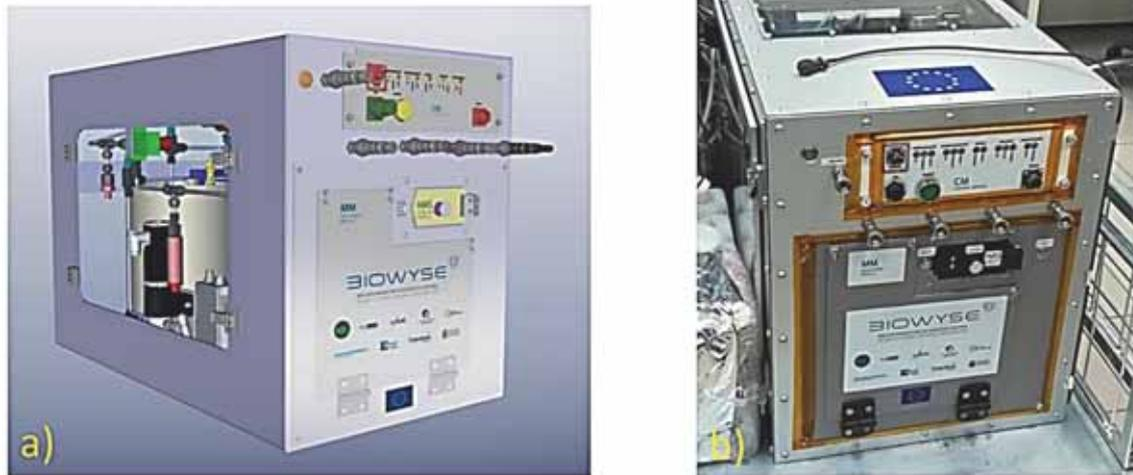
Fig. 3. BIOWYSE breadboard “as designed” a) vs “as built” b)
