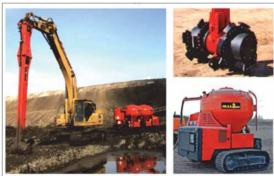
**Fig. 5.** Examples of full-scale in situ mixed amendments applications: STAMIX by Allu Stamix Oy (Allu Stamix, 2020)
