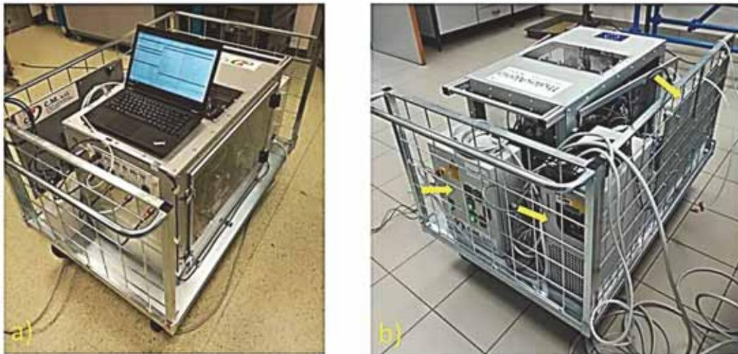
Fig. 9. BIOWYSE support equipment for field tests. a) PC tool, b) power supply, chiller and fluidic panel
