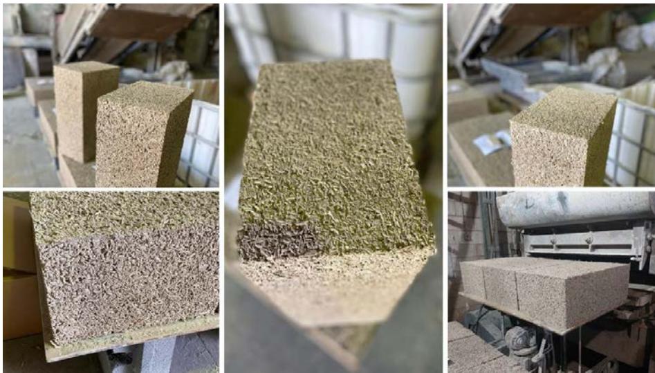
Fig. 1. Some images of the bio-block prototype produced and test (courtesy of PEDONE Srl)
