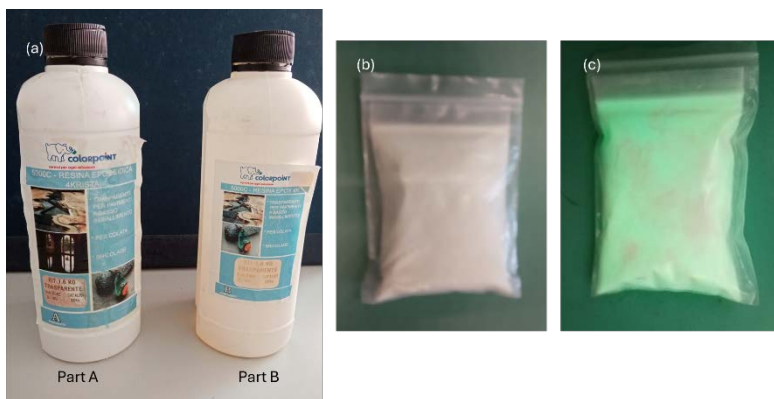
Fig. 3. (a) Epoxy system composed of resin (Part A) and hardener (Part B); (b) Photoluminescent powder; (c) Photoluminescent powder exhibiting visible luminous activity under light exposure
