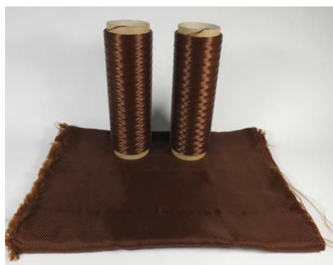
Fig. 1. Lignin yarn and woven fabric produced by DITF Denkendorf
