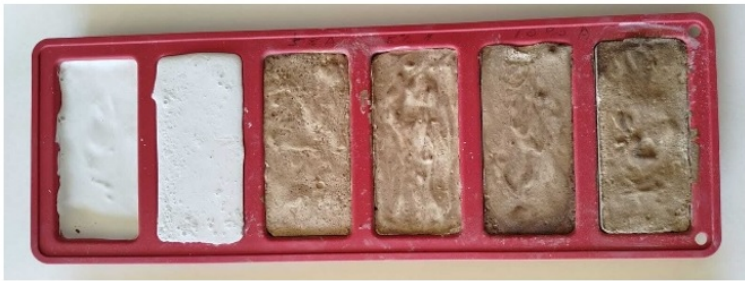
Fig. 3. Chalky matrix specimens with different SCG contents with silicone mold size (2.1x10.0 x 5.1) cm
