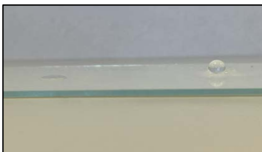
Fig. 7. Difference in wettability of an untreated (left) or aerogel-treated (right) glass surface
