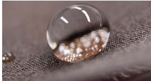
Fig. 3. Water drop on functionalized surface by DITF
