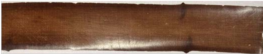
Fig. 2. Lignin film laminated on a cellulose woven fabric by DITF Denkendorf
