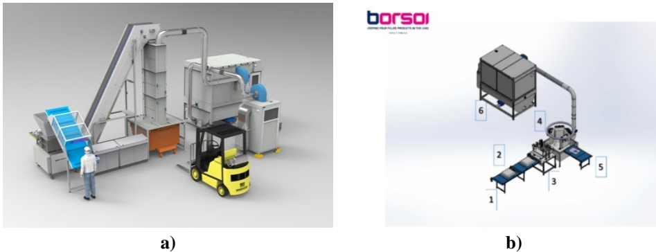
Figure 1. Borsoi's modular systems for recycling of padded textiles: (a) jackets and duvets; (b) mattresses, toppers, and pillows. The recycling workflow includes: 1. Loading Station (automated or with operator); 2. Loading Conveyor; 3. Compression and Cutting Unit; 4. Delayering, Emptying and Separation Unit; 5. Cover/Shell Discharge Conveyor; 6. Filling Collection Silo
