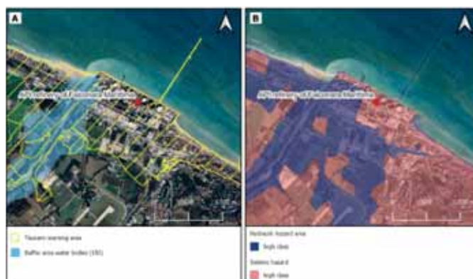
Fig. 2. Falconara Marittima refinery is A) in the water body buffer area and tsunami alert area and B) in the High hydraulic and seismic risk class
