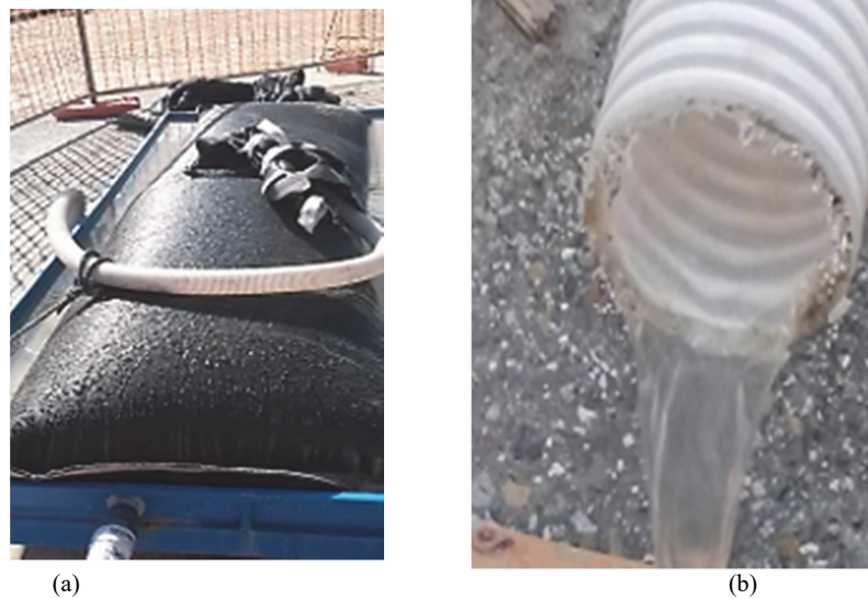
Fig. 4. Pilot plant filtration system: (a) Geo tube constructed and connected to the pipeline for feeding the polyelectrolyte–water mixture exiting the reactor; (b) discharge of clarified water after filtration through the geotextile
