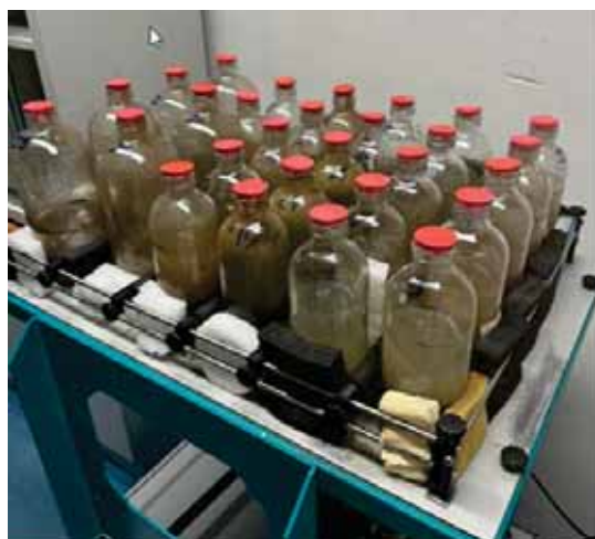
Fig. 6. Anaerobic digestion reactors on the orbital shaker
