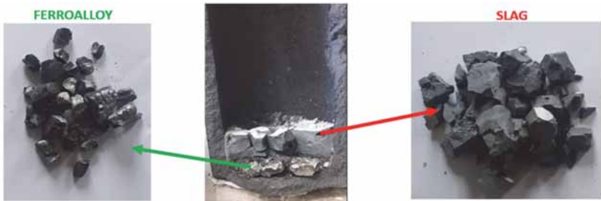
Fig. 7. Cross-section of the crucible coming from one experimental test
