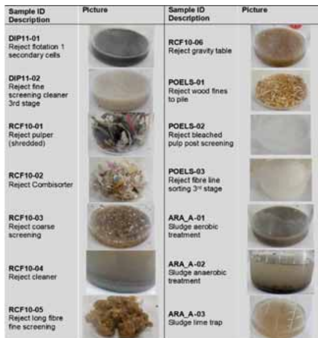
Fig. 3. List of wastes from Heinzelpaper production process, including ID, description and picture. The abbreviations mark the processes they come from: DIP = deinking process; RCF = recycled fiber; POELS = pulp from primary fibres; ARA = wastewater treatment
