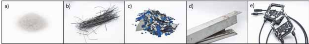
Fig. 5. Materials recovered in a 9-Tech demo plant that perform thermomechanical recycling from left to right: a) glass, b) copper ribbons, c) silicon PV cells, d) Aluminium, e) Junction boxes
